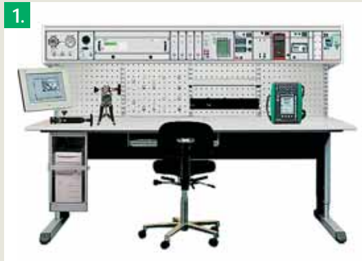
Pressure/Electrical Calibration workstation
