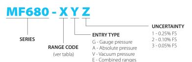
To include the barometric module, insert -B- between "series" and "range code". For electrical equipment only, include -E- without pressure range code.
